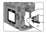
Before inserting or removing the CF memory card, turn the camera off.
