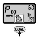
Together with image size, image quality determines the number of images that can be stored on the CF memory card. Press the **QUAL** button to choose an image-quality mode
